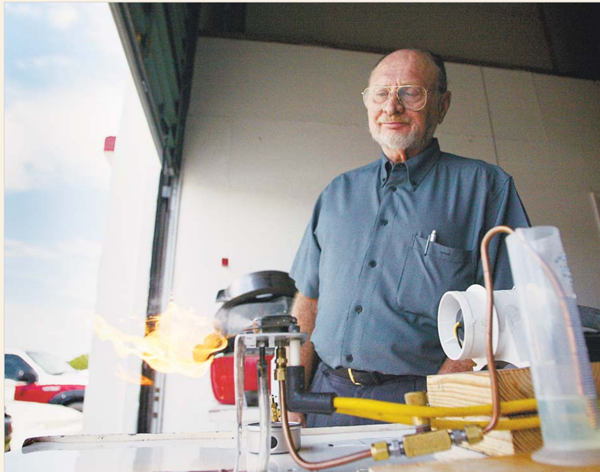
GREEN POWER: Inventor Harry Schoell demonstrates a fuel injection tester for his engine. "You can burn any combination of fuels all in the same container and it has no smell," Schoell says. Staff photos/Colleen K Cummins
